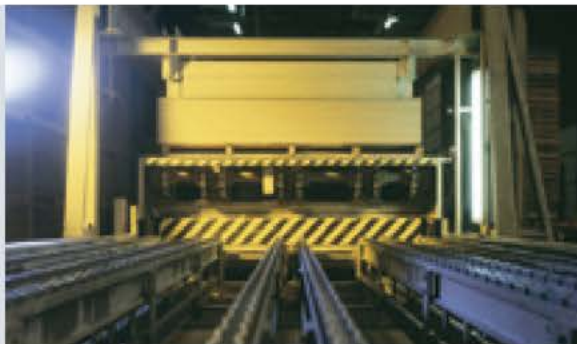
A finished raw board exits the dryer
