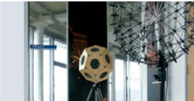
Dodecahedron loud speaker for measuring reverberation time
